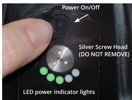
The power button and red/green LED indicator lights are located on the front of the elbow.
