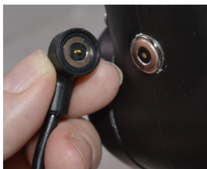
The charge port is located on the back of the elbow and connects with a break-away magnetic charging plug.
