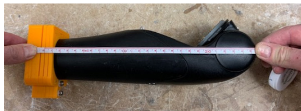
Fig 7. Measure length from the center of rotation.
