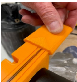
Fig 10. Cut through guide slot with a hack saw.
