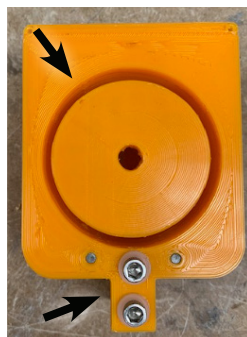
Fig 4. Circular disk groove to secure arm, and bottom tab for vice insertion.
