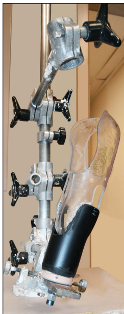
Figure 4 - Vertical Transfer Fixture with temporary alignment fixture fabricated from PVC.
