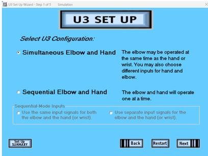
**Simultaneous vs. Sequential:** If using separate Hand and Elbow inputs, choose “Use separate input signals” and connect both inputs to the Wire Harness. If you choose “Use the same inputs,” the Elbow input will also be used for the Hand, when the elbow is locked.
