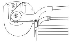
**6.** Slide damping ring over PEEK rods and then temporarily attach wrist unit.
