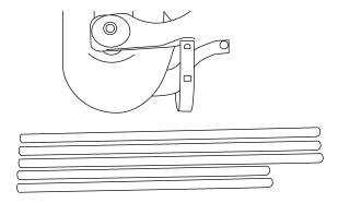
**5.** Place PEEK rods into saddle assembly and tighten attachment screws to 20 in·lb.
