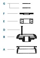
58700 OW-100LR with Laminating Ring 59526 Laminating Ring A. В. 58698 **Body Assembly** C. 52171 Bushing D. 52172 Cover E. 52173 Washer, 2 Each 70242 Screw, #8-32, 2 Each
