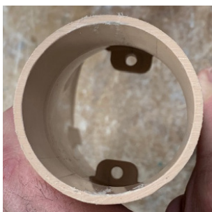
Fig 12. Deburr the edges and sand to smooth the cut end. Use caution with debris.
