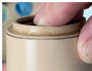
Fig 13. You should not see the O-ring when fully seated and glued in place.
