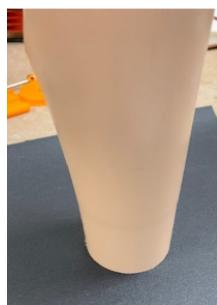
Fig 12. Deburr the edges and sand to smooth the cut end. Use caution with debris.
