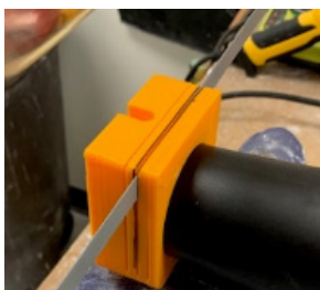
Fig 10. Cut through guide slot with a hack saw.
