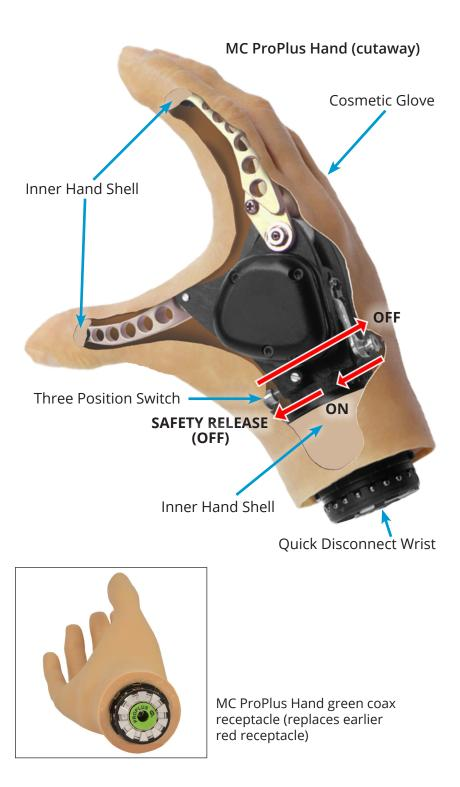
for the hand along with some moisture resistance. If a hole or damage is discovered, the hand shell should be replaced. Some smaller sized hands do not have an inner hand shell, they have only a cosmetic glove. This requires a special order from Motion Control.
