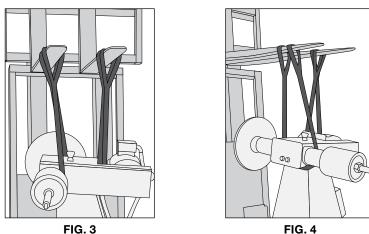
WARNING! Do not place the straps in any other positions such as around the shaft. Lifting or moving the machine by the shaft will damage the shaft and void the warranty. Failure to use proper lifting technique and strap location may result in permanent damage to the machine and/or serious injury to people who are near it.
